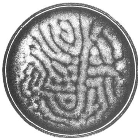
Plate 1. Spatial stationary pattern obtained by light irradiation of a saturated solution of mercury dithizonate. (Courtesy of Dr. J. C. Micheau.)
